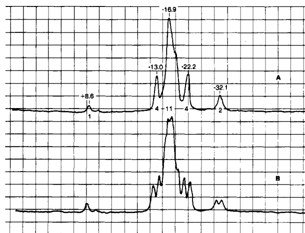
Figure 1. 80.5-MHz ^{11}B NMR spectrum of [(CH_3)_3NH]_2B_{22}H_{24} measured in acetone: (A) proton decoupled, (B) undecoupled. Chemical shifts [ppm, relative to BF_3 \cdot O(C_2H_5)_2 ] 23 are indicated. Relative areas appear beneath the peaks.
